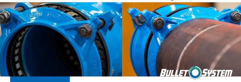
The BulletSleeve by Hawle is an all-in-one socket coupling used to join and restrain steel, DIP, PE/PVC, and AC pipes with corrosion protected connections. Adaptable to varying outside dimensions, ranging from 2- to 16-inches, with a bolt head locking device for one hand tightening. The reusable couplings are rated up to 250psi and carry a 10-year factory warranty. Reduces installation time and cost compared to a standard coupling.
